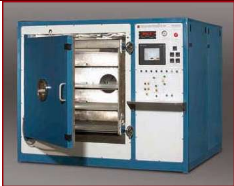
Above: Model PC 48 with optional heated shelves and standard PLC controller
