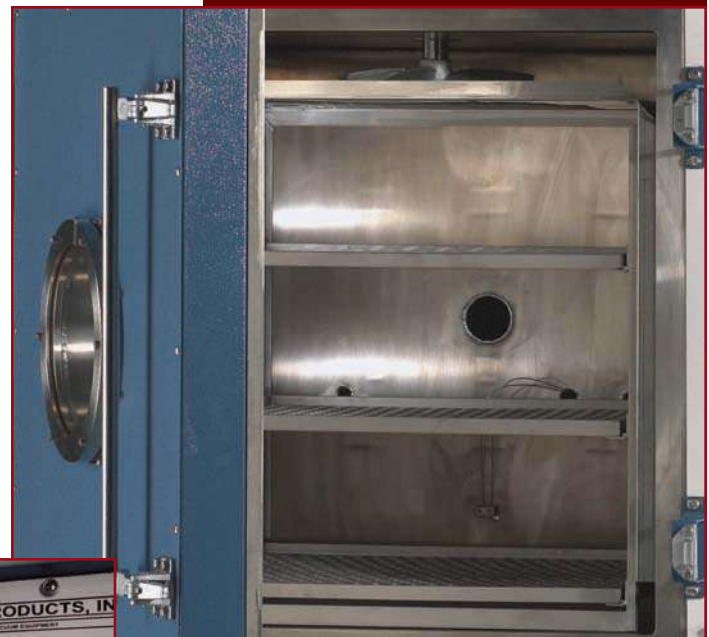
The photo detail above shows the all stainless steel chamber interior with inert gas stirring fan and removable sliding shelf configuration.
